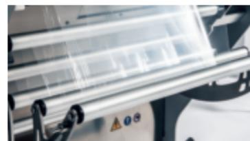
Optimised film unwinding and tensioning system
